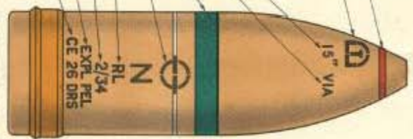
TYPICAL NOSE FUZED SHELL HE FILLED TNT
