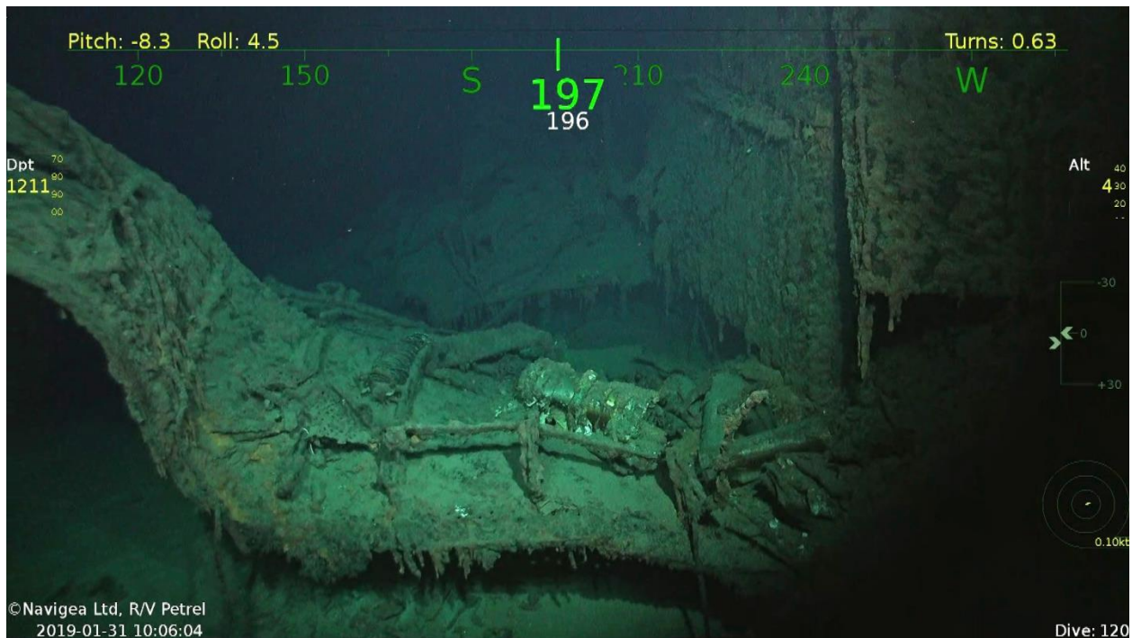
Figure 33 - Starboard hull break showing shattered hull
