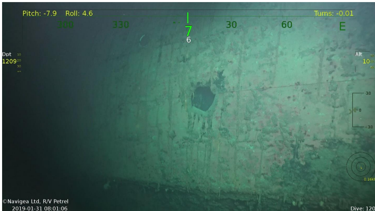
Figure 7 – 16-inch shell hit Frame 100 port side
