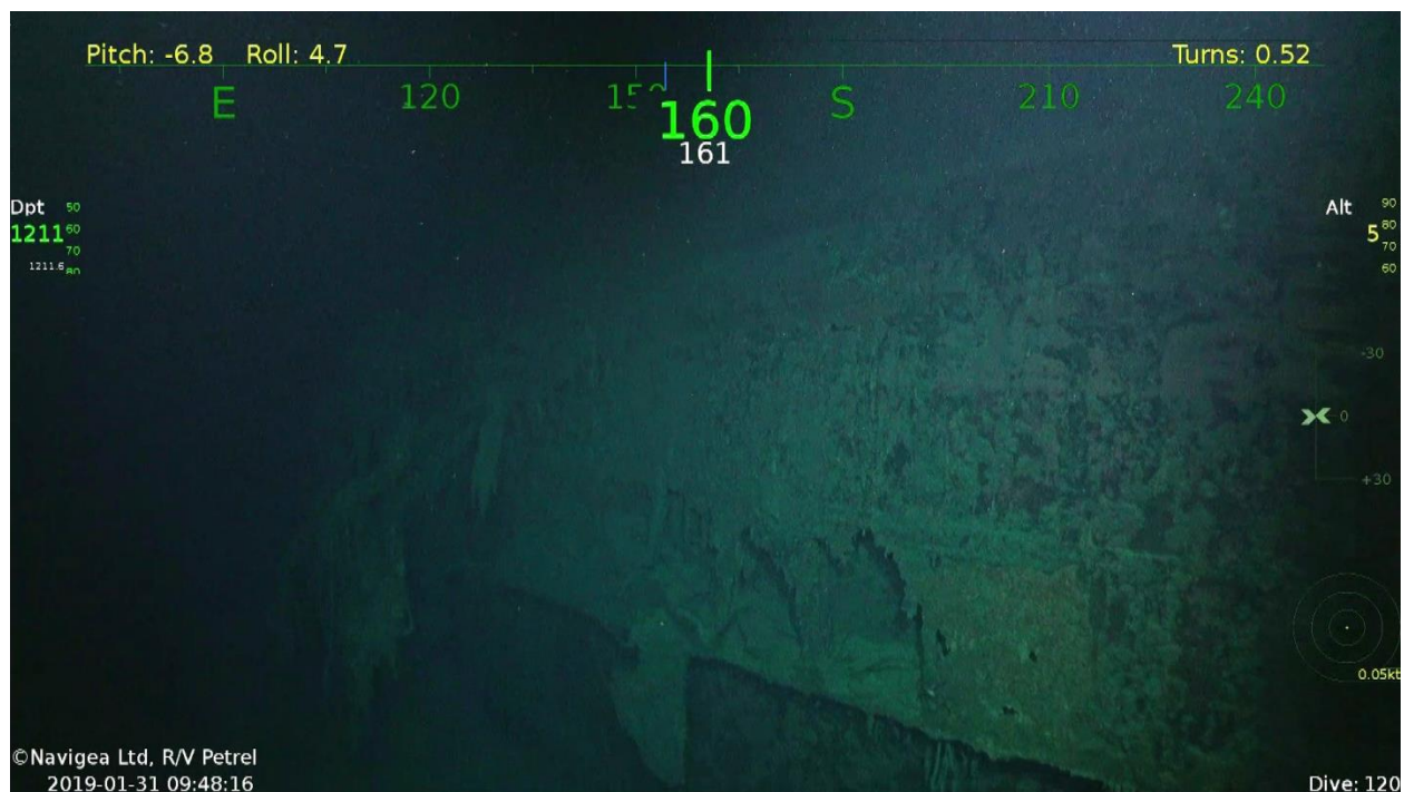
Figure 31 - Beginning of starboard hull break with hull shattered and peeled back from within
