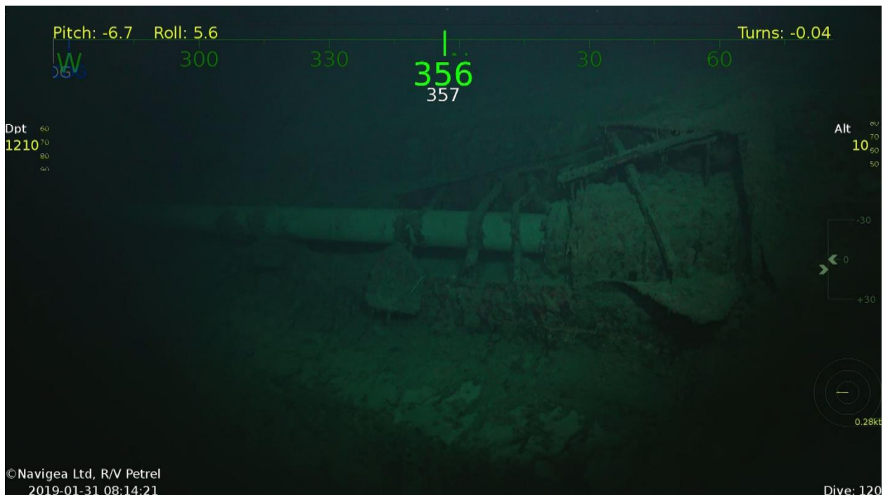
Figure 11 - Frame 258 outer port shaft shows blast damage as it enters her hull
