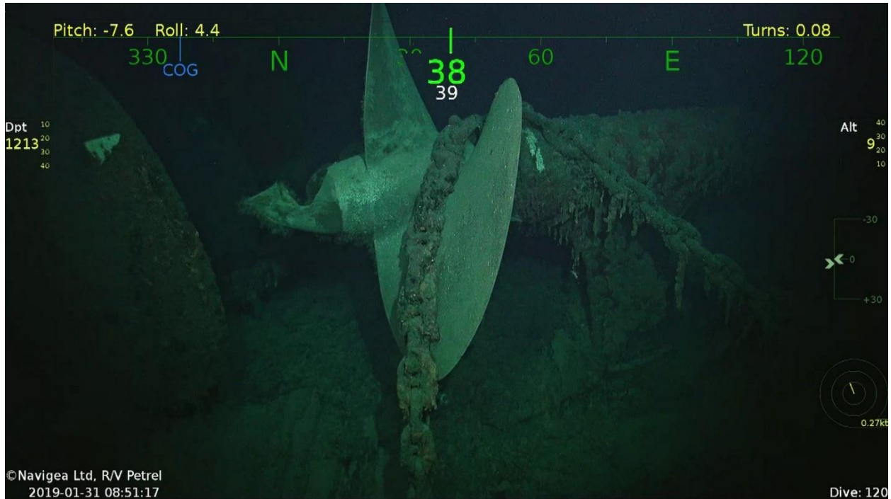
Figure 13 - Inboard port propeller is also undamaged
