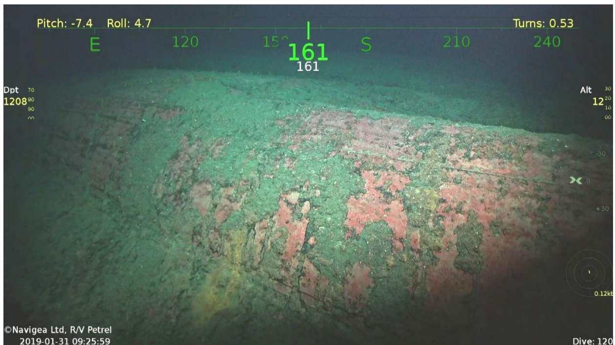
Figure 24 - Signs of implosion along Kirishima's keel
