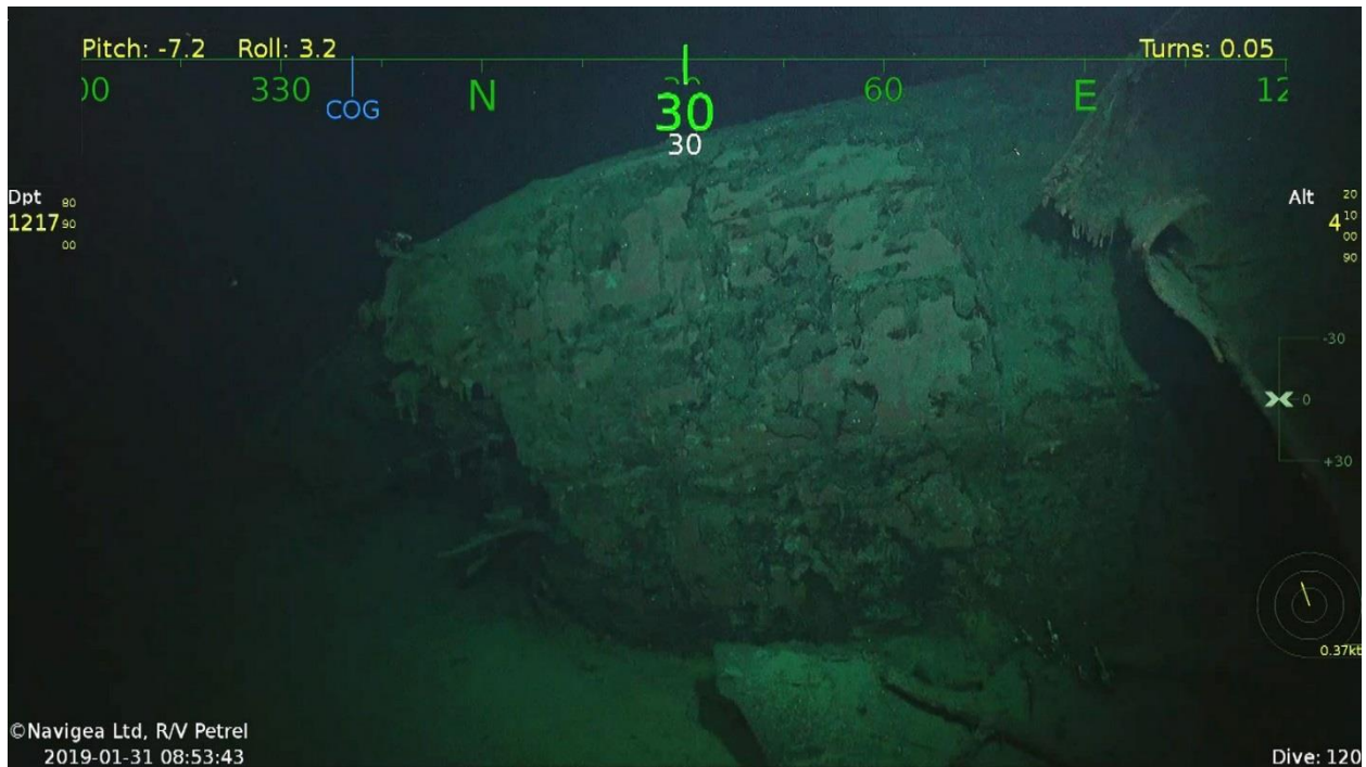
Figure 15 - Kirishima's stern with bent keel
